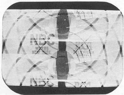
Figure 7—INCORRECT VERTICAL HOLD To correct—Adjust Vertical Hold Control until picture "locks in"
