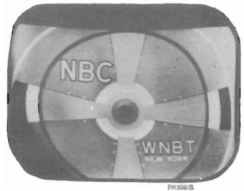
Figure 44—Focus Coil and Ion Trap Magnet Misadjusted
