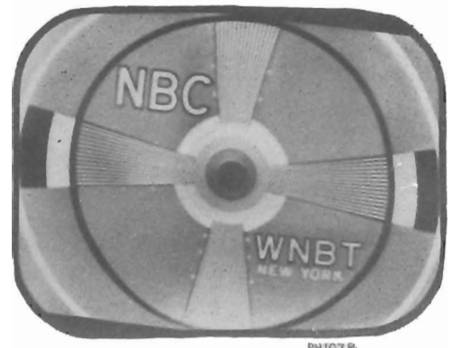
Figure 46—Deflection Yoke Misadjusted (Rotated)
