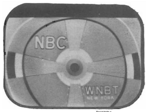
Figure 47—Horizontal Centering Control Misadjusted
