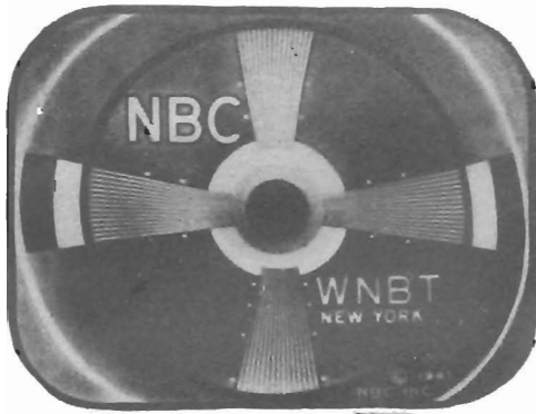
Figure 38—Brightness Control Misadjusted
