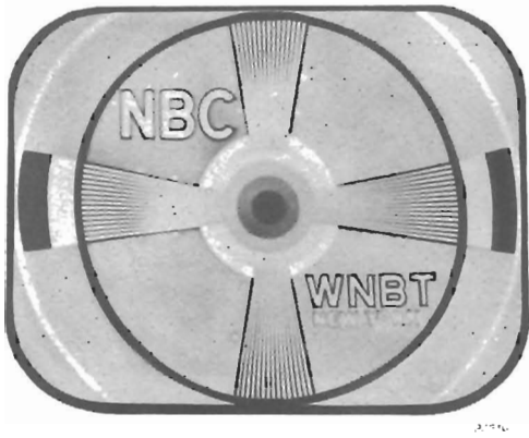
Figure 36—Vertical Hold Control Misadjusted
